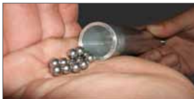
Pull the pounder out the holder and fill in the steel balls (not more than 12).
