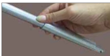
Insert the pounder carefully and the tool is ready for use. If too much pressure is applied, the balls are pressed out at the bottom at the tool. Handle with care!
